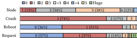
**Figure 3: Basic input conditions.** It shows the minimum numbers of nodes, crashes, reboots and client requests required by the 103 crash recovery bugs. *H* means a large number, e.g., 1000.
