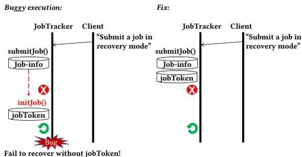
Figure 5: Incomplete fix for bug m5169. The left part shows the buggy execution. The right part shows the fix.
